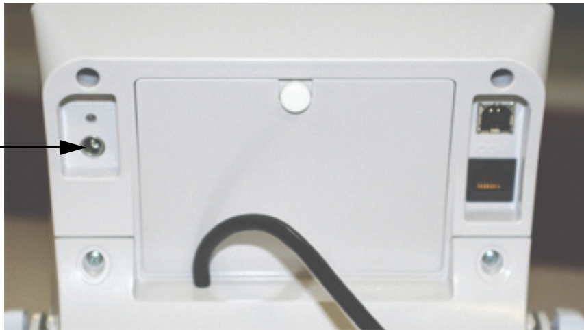
Figure 4-5. Power Connection Site
