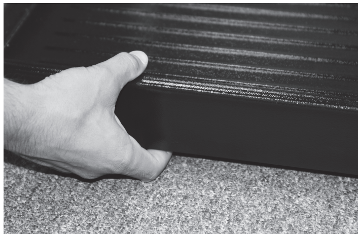
Figure 3-2. Have a Minimal Amount of Clearance Between the Scale Base and the Floor
