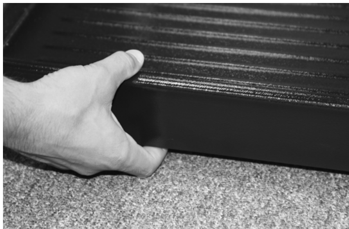
Figure 3-5. Have a Minimal Amount of Clearance Between the Scale Base and the Floor
