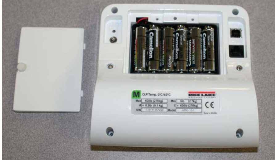
Figure 3-15. Batteries in Battery Chamber
