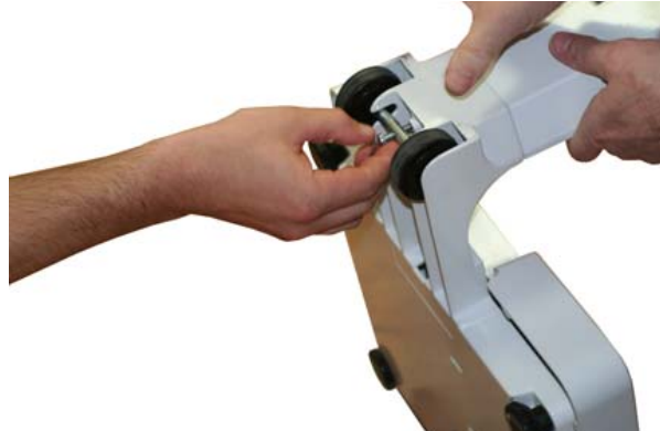
Figure 3-4. Attach Wheel Assembly
