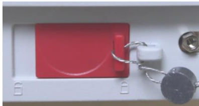
Locked with Wire Seal
