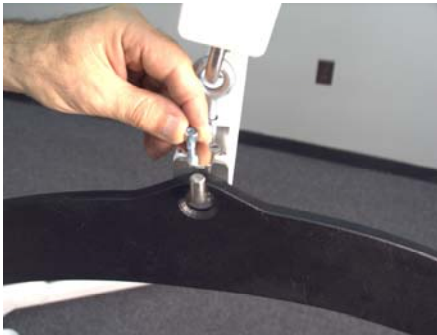
Lift hoop slightly to ease screw installation
