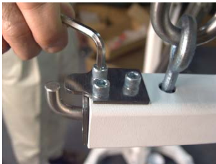
Remove outer 2 Screws Loosen inner Screw
