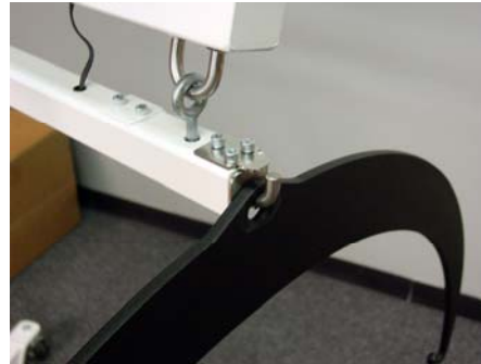
Completely tighten all three retainer plate screws
