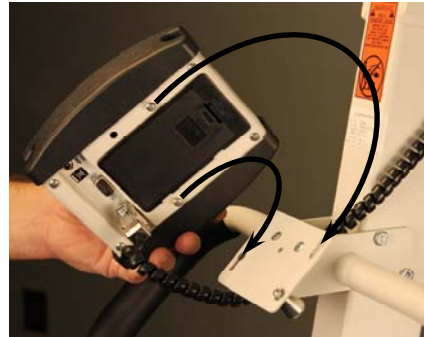
Align screw heads with large end of slotted holes and pull down to secure indicator
