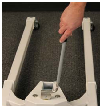
Install Handle Extension
