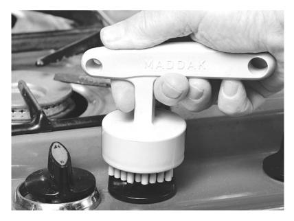
Push the pins of the TKO<sup>™</sup> against the knob/handle. The pins in contact with the highest points of the knob/handle will depress while the others remain extended. The extended pins engage the sides of the knob/handle so that it turns when the TKO<sup>™</sup> handle is twisted.
